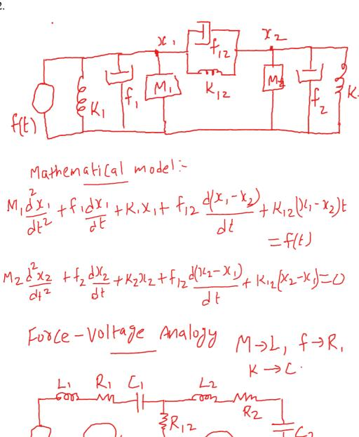
$$\frac{L_{1}di_{1}}{dt} + R_{1}i_{1}(t) + \frac{1}{C_{1}} \int i_{1}(t)dt + R_{1}i_{1}(t-i_{2})t dt = Q(t)$$
