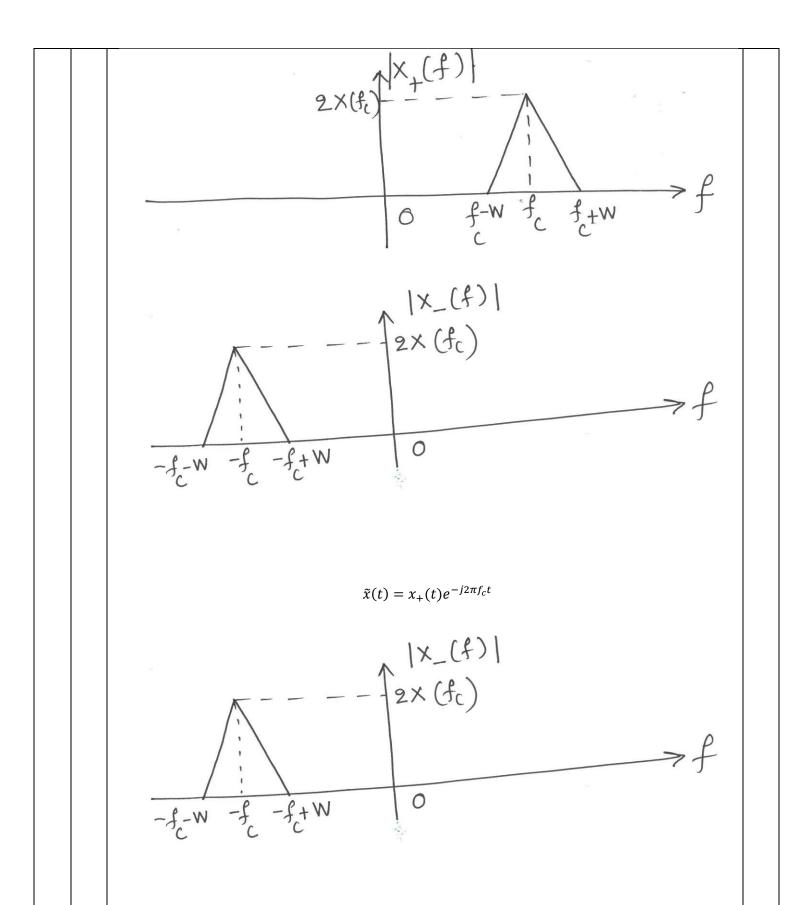
Derive an expression for the canonical representation of bandpass signals. Obtain a scheme for extracting in-phase and quadrature components of bandpass signals. Draw the corresponding block diagram.
