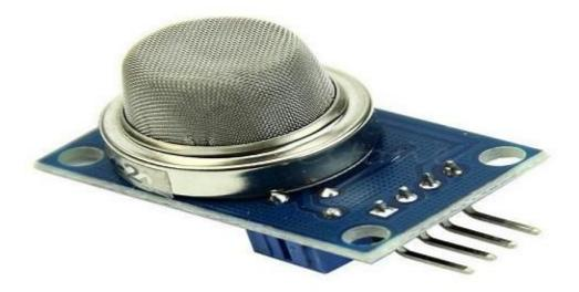
MQ2 is a metal oxide semiconductor type gas sensor. Concentrations of gas in the gas is measured using a voltage divider network present in the sensor. This sensor works on 5V DC voltage. It can detect gases in the concentration of range 200 to 10000ppm. Working Principle
