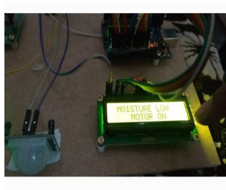
Fig22: Moisture low and motor on display
