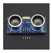
Ultrasonic Sensor (The HC-SR04 Ultrasonic Distance Sensor is a sensor used for detecting the distance to an object using sonar).
