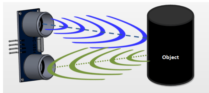
Figure 4.3 Diagram of the basic ultrasonic sensor operation
