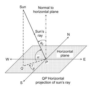
(c) Surface Azimuth angle: ( $\gamma_s$ ) It is the angle on a horizontal plane, between the line due south and the projection of sun's ray on the horizontal plane. It is taken as positive when measured from south towards west.
