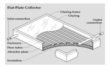
In steady state, the performance of a solar collector is described by an energy balance that indicates the distribution of incident solar energy into useful energy gain, thermal losses, and optical losses.
