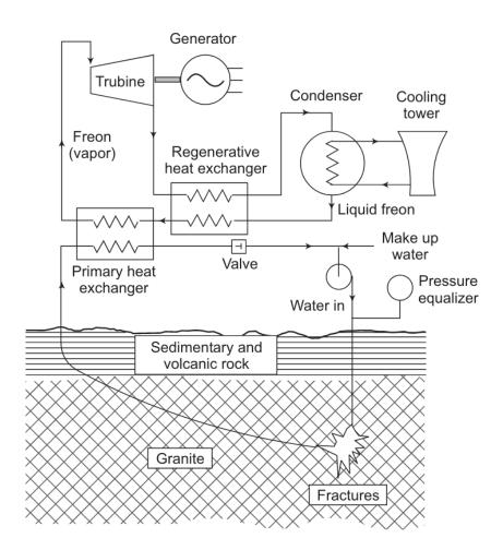
There are regions underground at temperatures exceeding 200 °C, with little or no water. The rocks are impermeable and/or there is no surface water in the vicinity. Such resources up to a depth of 5 km are estimated to be significant and worthy of development as a source of energy. Hot dry rocks
