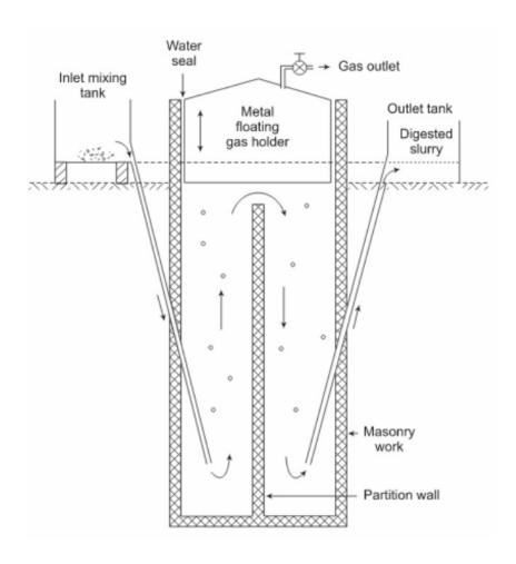
KVIC Biogas Plant: It has an inverted mild steel drum to work as gasholder. This is the most expensive component of the plant. The drum floats either direct on fermentation slurry or in a water jacket of its own. Most Indian plants now have a pair of central guide pipes.
