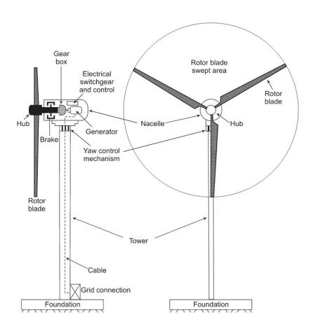
Main Components: The constructional details of most common, three-blade rotor, horizontal axis wind turbine are shown in figure above.
