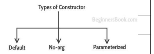
**Default constructor:** If you do not implement any constructor in your class, Java compiler inserts a default constructor into your code on your behalf. This constructor is known as default constructor. You would not find it in your source code(the java file) as it would be inserted into the code during compilation and exists in .class file. This process is shown in the diagram below:
