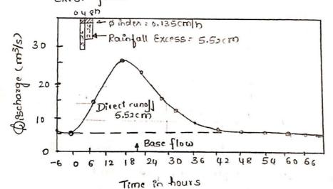
Area of DRH =  $(6 \times 60 \times 60) \left[ \frac{1}{2} (8) + \frac{1}{2} (8 + 21) + \frac{1}{2} (21 + 16) + \frac{1}{6} (16 + 11) + \frac{1}{2} (11 + 7) + \frac{1}{2} (7 + 4) + \frac{1}{2} (4 + 2) + \frac{1}{2} (2) \right]$
