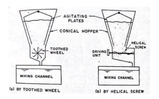
regulated by toothed wheel or a helical screw. The speed of the toothed wheel or helical screw is turn controlled by connecting it to a venture device installed in the raw water pipes bringing water to the mixing basin. The quantity of the coagulant released is, thus controlled in proportion to the quantity of raw water entering the mixing tank.
