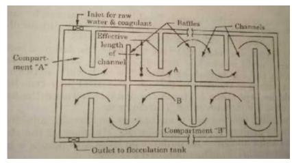
vertically over and under the baffles. The hinderness and disturbances created by the provision of baffles in the path of flow, give it sufficient agitation, as to cause necessary mixing to develop the floc. 2) Mixing Basin Equipped with Mechanical Devices: most of the
