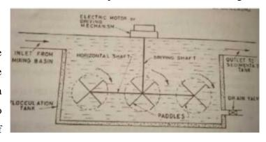
the floc particles. Therefore, from the mixing basin the water is taken to a flocculation tank called a flocculator, where it is given a slow stirring motion. Rectangular tanks fitted with paddles operated by electric motors can best serve this purpose.
