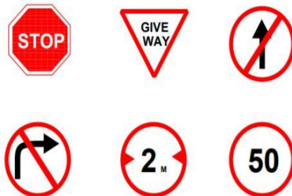
Figure: Stop sign, give way sign, signs for no entry, sign indicating prohibition for right turn, vehicle width limit sign, speed limit sign
