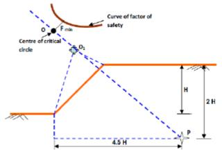
2(c) An embankment is to be constructed with a soil having C=20 kN/m²,  $\phi$ = 10° and  $\gamma$ =19 kN/m³. The desired factor of safety with respect to cohesion as well as friction is1.5. Determine (1) safe height of the desired slope if slope is 2H to 1V (2) Safe angle of slope if the desired height is 15m. For  $\phi$ =10° Taylor's stability numbers are as follows:
