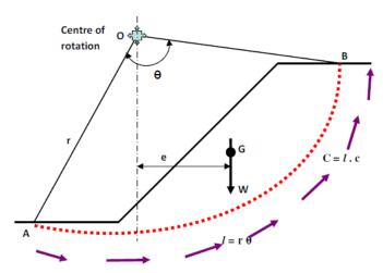
Let AB be a trial slip surface in the form of a circular arc of radius 'r' with respect to center of rotation 'O' as shown in figure above. Let 'W' be the weight of the soil within the slip surface. Let 'G' be the position of its centre of gravity.
