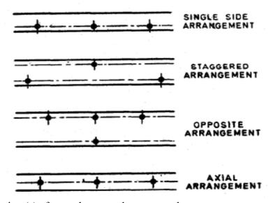
Spacing (s) of street lamp can be computed as  $s = \frac{\text{Lamp lumen} \times \text{coeffecient of utilization} \times \text{Maintenance factor}}{\text{average flux} \times \text{width of the road}}$
