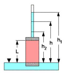
Total head **h** in standpipe of area **a** is allowed to fall. Hydraulic gradient varies with time. Heads **h1** and **h2** are measured at times **t1** and **t2**. At any time **t**, flow through the soil sample of cross-sectional area **A** is
