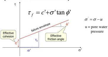
$\tau_{\text{f}}$  is the maximum shear stress the soil can take without failure, under normal effective stress of  $\sigma^{\prime}.$
