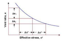
In the arithmetic plot as shown, as the soil compresses, for the same increase of effective stress Ds', the void ratio reduces by a smaller magnitude, from  $De_1$  to  $De_2$ . This is on account of an increasingly denser packing of the soil particles as the pore water is forced out. In fine soils, a much longer time is required for the pore water to escape, as compared to coarse soils.
