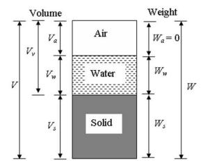
**Void ratio** (e) is the ratio of the volume of voids  $(V_v)$  to the volume of soil solids  $(V_s)$ , and is expressed as a decimal.
