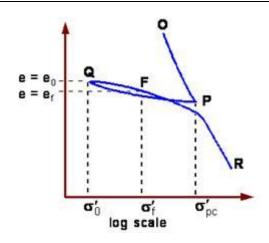
OP corresponds to initial loading of the soil. PQ corresponds to unloading of the soil. QFR corresponds to a reloading of the soil. Upon reloading beyond P, the soil continues along the path that it would have followed if loaded from O to R continuously.
