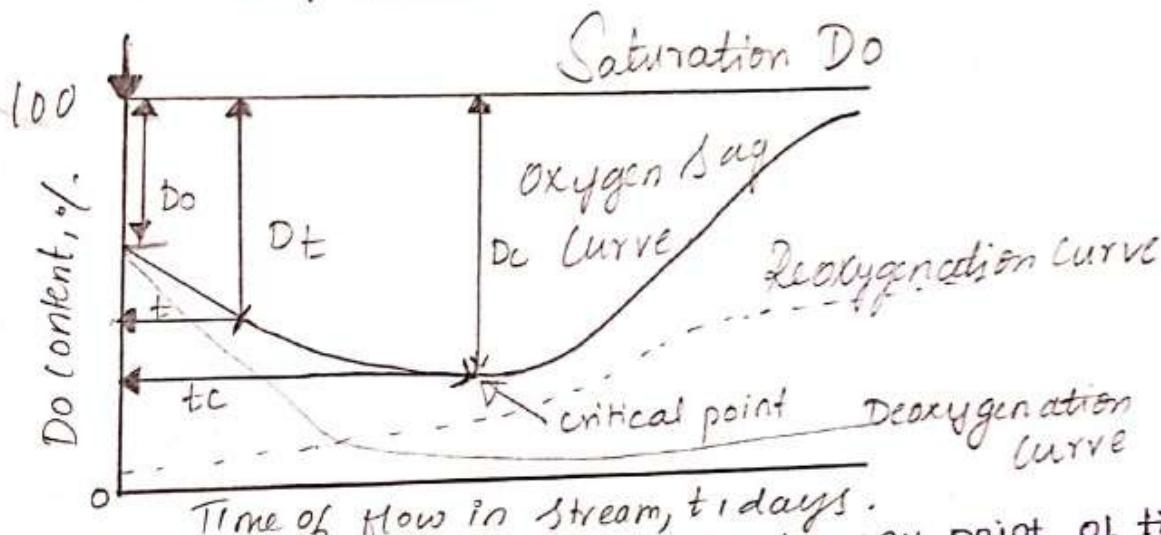
The oxygen sag in the stream at any point of time during self purification process is the difference b/w saturation DO content and actual DO content. The amount of resultant oxygen deficit can be obtained by algebraically adding the deoxygenation and re-oxygenation curves. This curve is called as oxygen sag curve.
