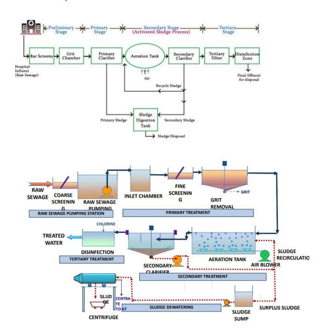
Pumping Station • Receiving Chamber • Coarse Screening • Wet Well (Raw Sewage Sump) • Pump House • Raw Sewage Pumps.
