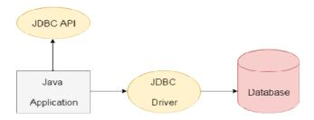
JDBC Driver is a software component that enables java application to interact with the database.
