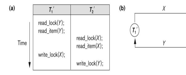
Illustrating the deadlock problem. (a) A partial schedule of  $T_1$  and  $T_2$  that is in a state of deadlock. (b) A wait-for graph for the partial schedule in (a).
