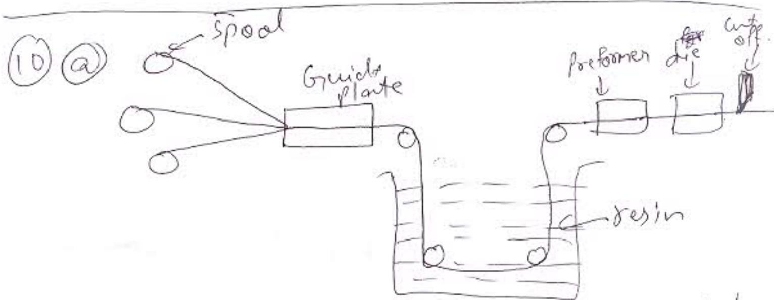
Fibers from different spools are guided into the resin bath and then preformed by heating it then its pulled through a die ~~re~~ with the help of rollers and then cut off at required lengths.
