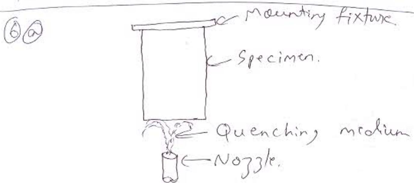
The sample is first austenitized then placed in the fixture, then <sup>its subjected to</sup> a spray of uniform flow rate. Now the specimen cools at different rates the the sections of the specimen is taken then tested with rockwell hardness test.
