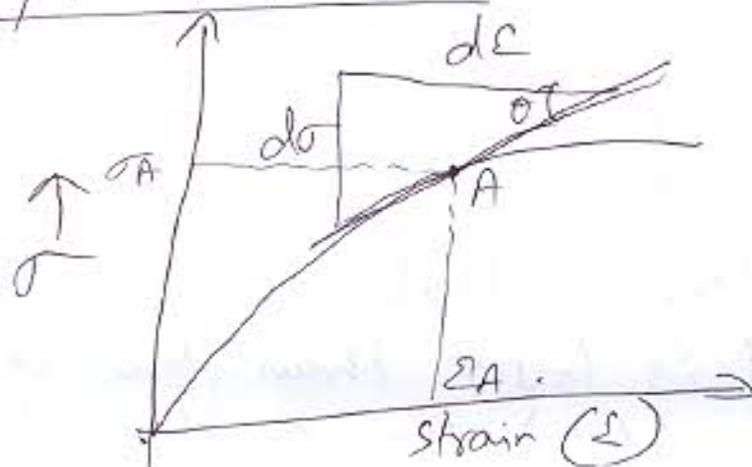
When the non-linearity of the curve is too high, tangent modulus is used. (6)
