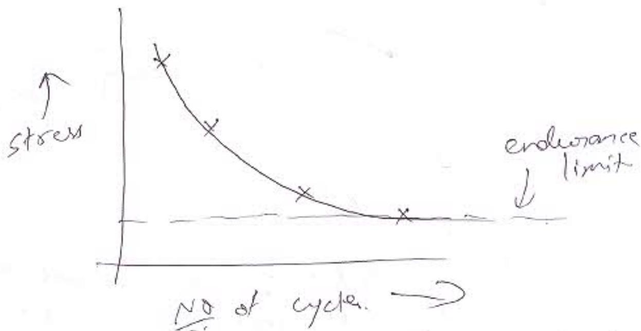
The above diagram represents a typical S-N curve. This curve is plotted to represent the experimental data obtained from fatigue testing. As the stress level is higher, the sample fractures at a lower no of cycles but as the stress level on the sample reduces, the no of cycles to failure increases. Once the stress level is lower than the endurance limit (for ferrous metals), the sample will not fracture.
