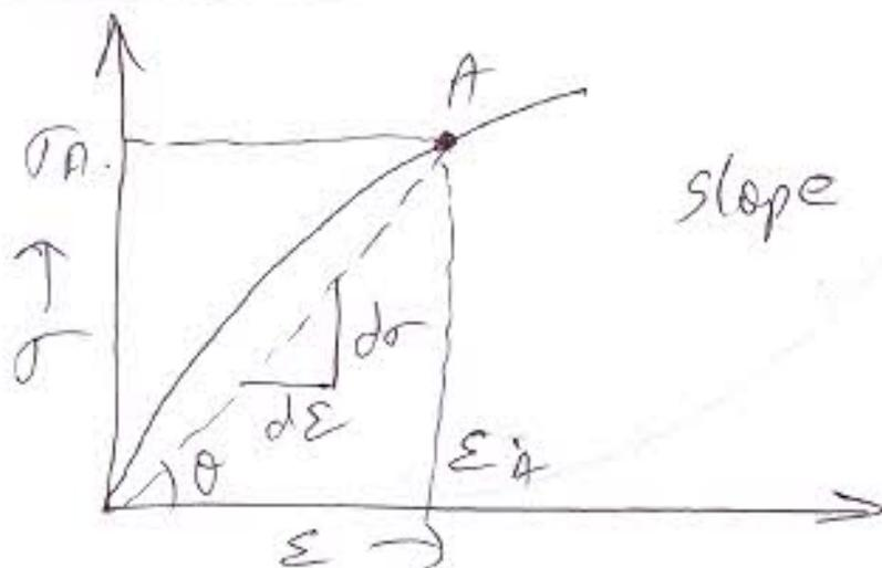
$$\text{slope} = \frac{d\sigma}{d\varepsilon} = \text{secant modulus}$$
