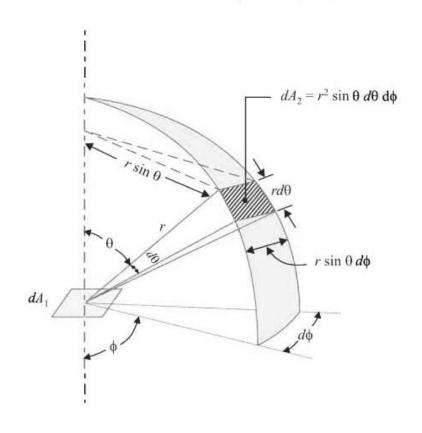
The fig shows a small black surface of a read A, emitting radiations in different directions. A black body radiation collector through which the radiation pass is located at an angular position characterised by zonith angle 0 towards the surface normal 4 angle 0 of a spherical co-ordinate system. The collector substants a solid angle dw when veiwed from a point on the emitter.
