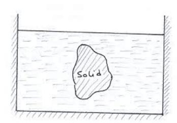
Consider a solid suddenly immersed in a well stirred fluid maintained at a uniform temp To.
