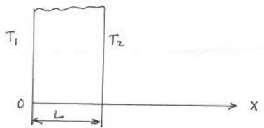
The specified temperature can be constant (steady state heat conduction) on may vary with time.
