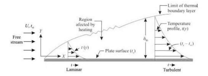
Inherever flow of fluid takes place past a heated on cold surface, a temporature field is set up in the vicinity of the surface. If the surface is notter than the fluid, the temporature distribution will be shown as In the above fig. The zone on this layer where in the temporature field exists to collect as thermal boundary layer.
