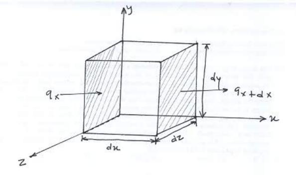
Consider a small rectangular element of dimensions du, dy +dz in x, y + z directions respectively.
