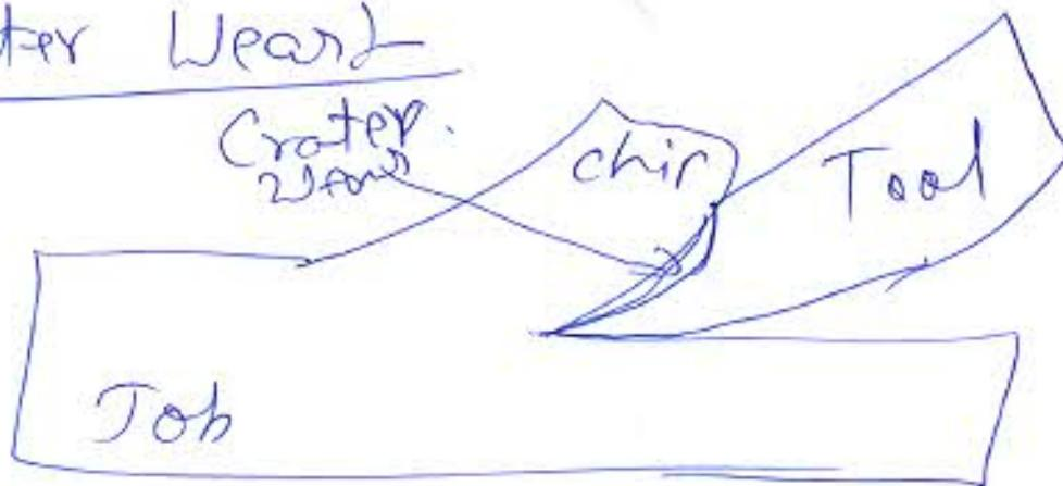
It is essentially the ~~to~~ erosion of an area on the tool face as shown in Fig above. It occurs when m/c ductile materials.
