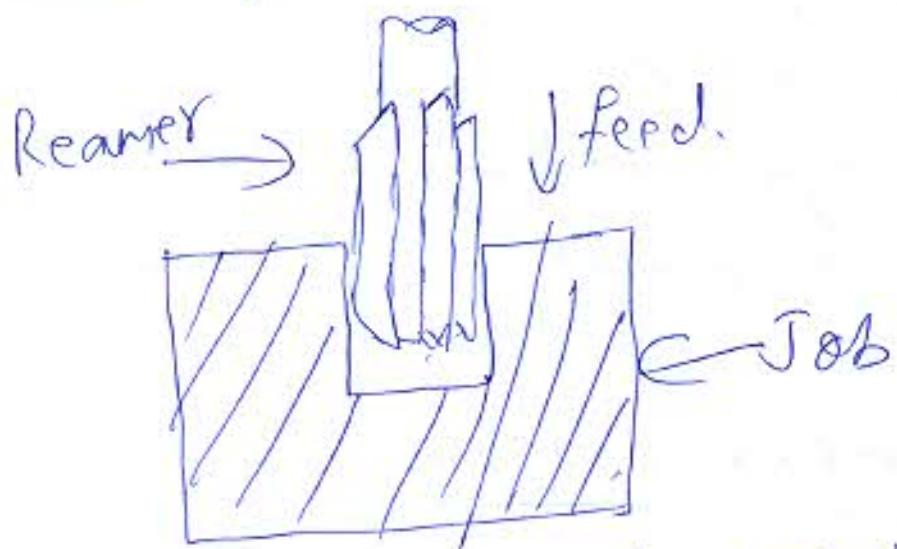
Reaming is an operation carried out for finishing a pre-drilled hole. The reamer rotates along the drill axis and the feed is parallel to the axis. The reamer has cutting edges running the entire length of the tool. This tool removes only small amounts of material but it gives a good surface finish to the inner walls of the previously drilled hole.
