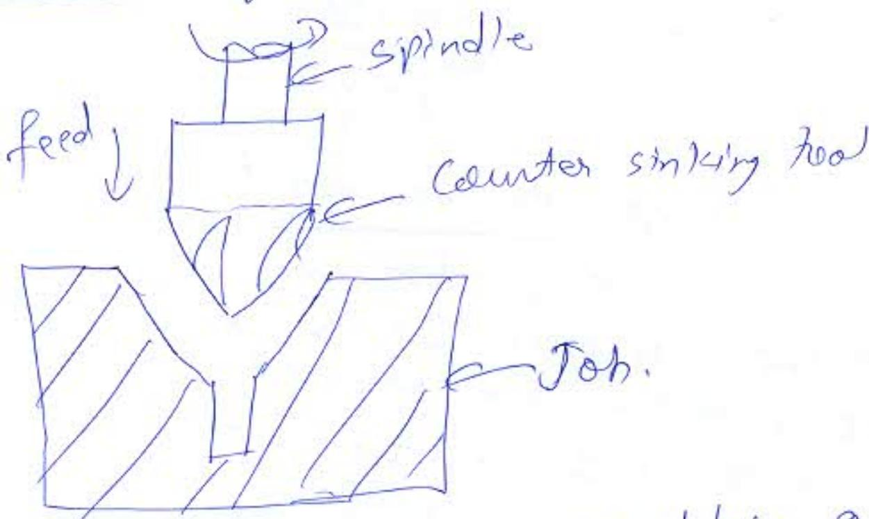
Counter sinking is done to obtain a tapered at the beginning of the previously drilled hole. As the rotating tool enters the drilled hole, because of the conical shape of the tool, it produces a taper at the
