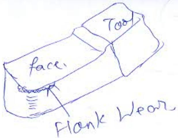
It is a form of wear which appears on the flank below the cutting edge of the tool. It's caused because of abrasive action b/w flank of the tool & the newly m/c surface.
