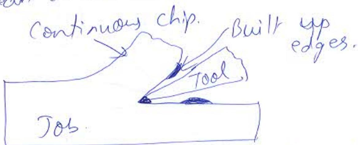
When machining tough steels such as alloy steels, toolsteels etc, larger cutting forces are required and this in turn produces a lot of heat at the tool-work interface. The high heat generated causes compressed metal adjacent to the tool nose to get welded to it in the form of metal lumps called built up edges.
