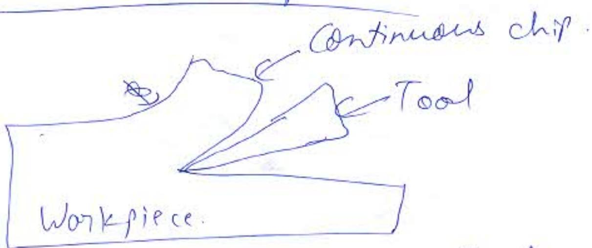
When the job is ductile fracture will not occur in the shear plane and the chip comes off in the form of long string or ribbon, with smooth shining surface.
