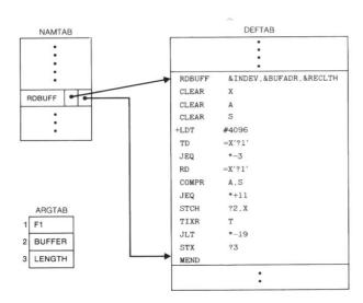
In fig 4.4(a) definition of RDBUFF is stored in DEFTAB, with an entry in NAMTAB having the pointers to the beginning and the end of the definition. The arguments referred by the instructions are denoted by their positional notations. For example, TD = X'?1'
