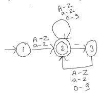
1)4Beta - Not recognized 2) hello\_5 - Recognized 3)hello10 - Recognized 4) alpha2beta - Recognized 5) alpha\_\_ 3delta - Not recognized 6) charlie5\_ - Not recognized 7)Charlie\_detlat2 - Recognized 8)abccccab - Recognized 9)r0123abc - Recognized 10)34abc - Not recognized
