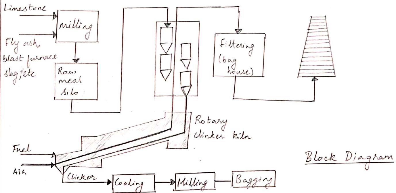
The first stage of cement production process is the sintering of a controlled mixture of raw materials in a kiln, typically a horizontal rotary kiln at temperature of  $\approx 1450^{\circ}\text{C}$ .
