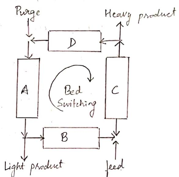
Simulated moving bed using cascaded fixed beds.
