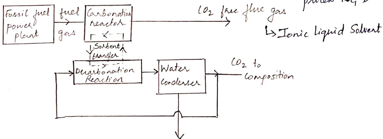
The dry sorbent process is illustrated in the above diagram.
