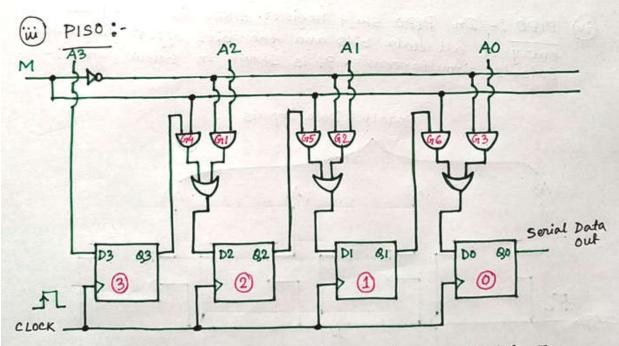
In this type, the bits are entered in parallel. The above Figure shows a 4 bit parallel in serial out shift negister.
