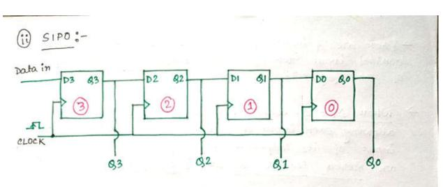
In this case, the data bits are entered into the Register in the same manner as discussed for the case of SISO. But the outputs are collected in parallel. Once the data are storted, each bit appears on its nespective output line and all the bits are available simultaneously.
