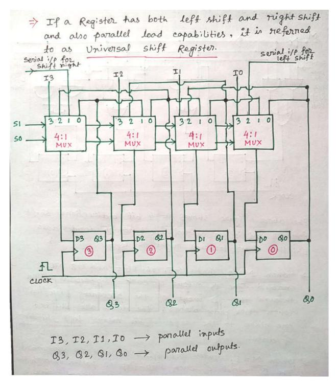
→ 9+ consists of 4 flipflops and 4 Multiplexers. The four Multiplexers have two common select inputs 51 and So. and they select appropriate input for D flip-flop. The below table shows the negister operation depending on the select lines of multiplexer.
