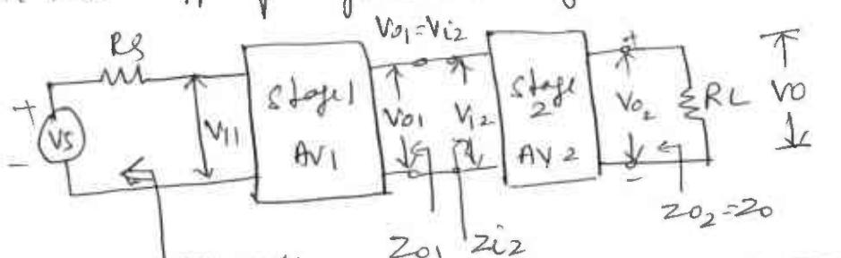
$A_V = \frac{V_{o2}}{V_{i1}} = \frac{V_{o2}}{V_{i2}} \frac{V_{i2}}{V_{i1}}$ $\therefore A_V = A_{V1} A_{V2}$ | <span style="float: right;">6 Marks</span><br><span style="float: right;">(3 M)</span><br><span style="float: right;">(3 M)</span> |
