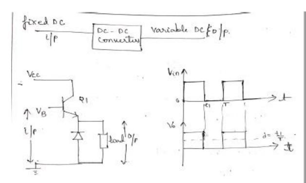
The DC to DC converter uses are BJT to regulate the O/r.
