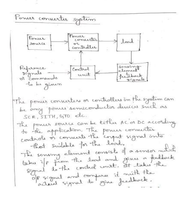
The control unit receives the feedback signal, makes a comparison to the desired signal. The steps to be taken if there is any error is carried out by the control unit.
