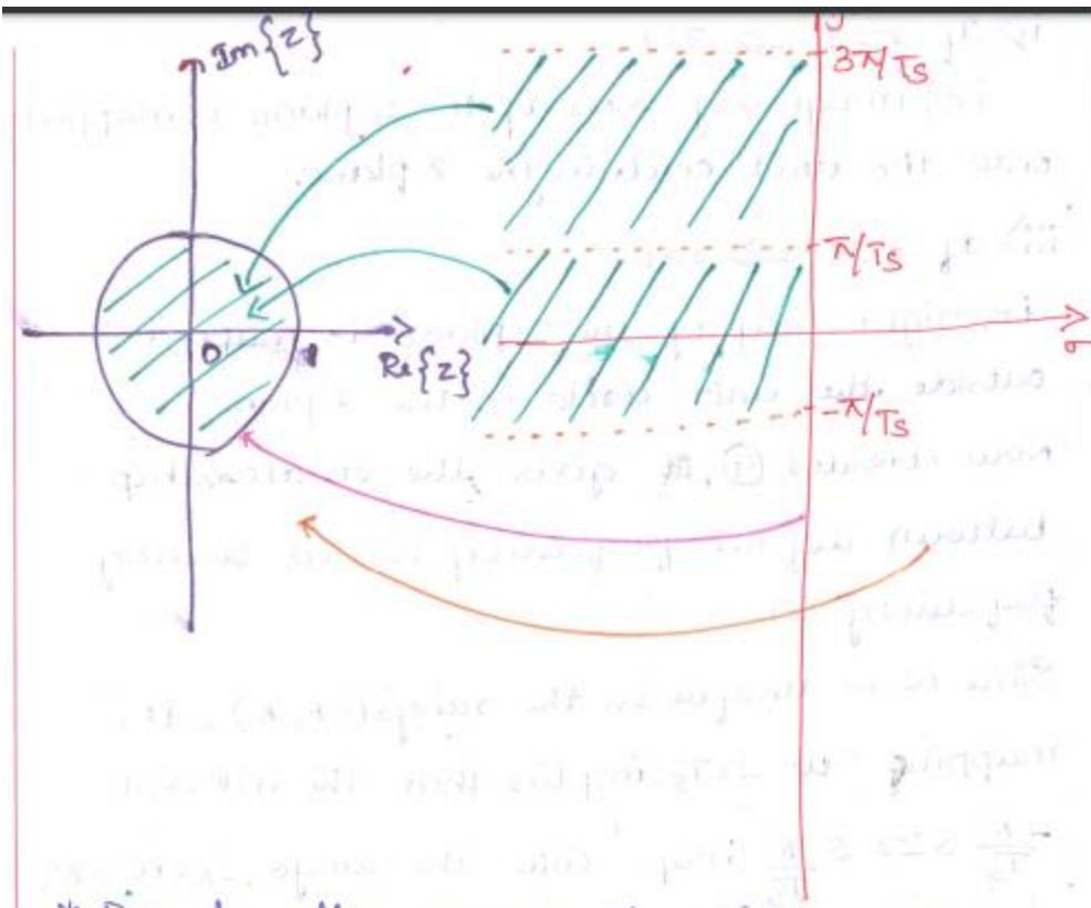
\* Due to the presence of aliasing, the impulse invariant method is appropriate for the design of lowpass & bandpass filters only. It is not suitable for high pass filters.
