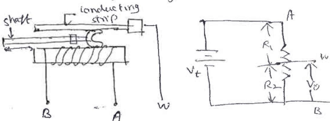
The output voltage depends on the wiper position & is therefore a function of the shaft position. This voltage may be applied to a voltmeter calibrated in cms for visual display.
