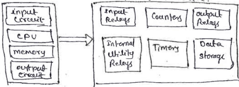
Input Relays: These are connected to the outside world. They physically exist & receive signals from switches, sensors, etc.
