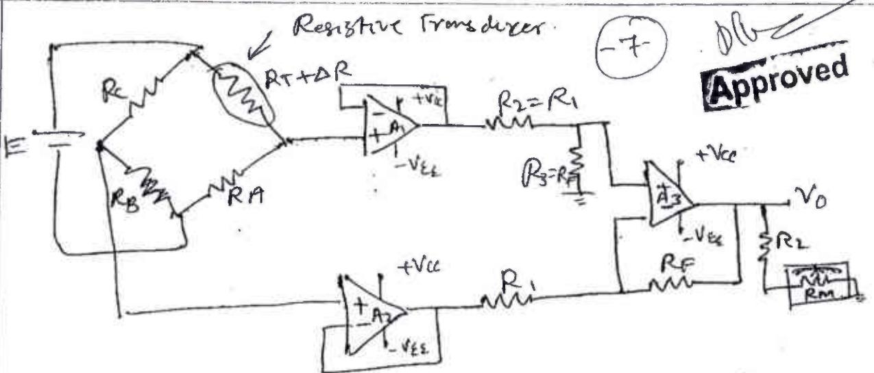
Initially the bridge is balanced at a desired reference condition. As the physical quantity to be measured changes, the resistance of the transducer also changes, causing the bridge to be unbalanced. Hence the 'off' voltage of the bridge is a function of the change in the resistance of the transducer.
