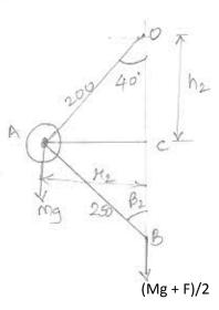
Given: OA = 200 mm = 0.2 m; AB = 0.25 m, M = 15 kg, M = 2 kg; F = 24 N;  $\alpha_1 = 30^\circ$ ,  $\alpha_2 = 40^\circ$
