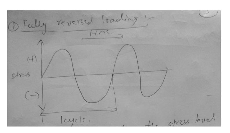
In this type of loading the stress had is taken to one extreme find of the spectrum and then it is reversed completly to the other side of the spectrum to the same magnitude side of the spectrum to the same magnitude Egt Rotating shafts. 1) Repeated loading/ time In this type of loading the material is subjected to a max stress and then reduced to a minimum stress but of the some nature This can be either tensile of compressive in This can be either operate within this enoclop.
