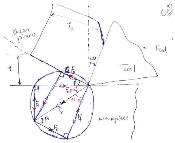
Let, de= Rake angle 1 el-oar angl of = Shear angle Friction force along the tool face.
