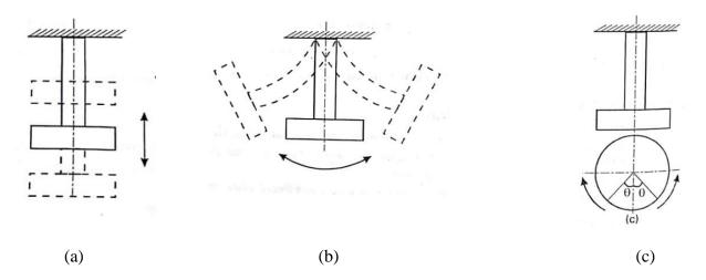
When the particles of the shaft or disc moves approximately perpendicular to the axis of the shaft, then the vibrations are known as transverse vibrations and is shown in Figure (b).
