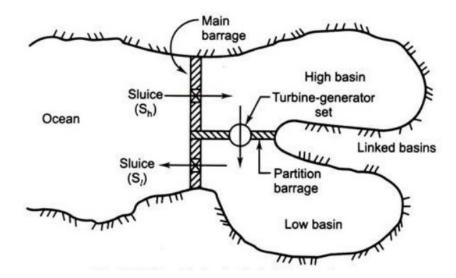
It requires two separate but adjacent basins. In one basin called "upper basin" (or high pool), the water level is maintained above that in the other, the low basin (or low pool). Because there is always a head between upper and lower basins, electricity can be generated continuously, although at a variable rate.
