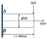
6. For the member shown below, the maximum shear stress induced at point B (in MPa) will be:
