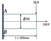
7. For the member shown, the value of maximum and minimum principal stress (in MPa) at point A is:
