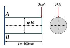
3. For the member shown in the figure, the maximum principal stress induced at point A will be (in MPa)
