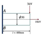
5. For the member shown below, the maximum shear stress induced at point A (in MPa) will be:
