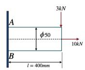
4. For the member shown in figure, the maximum principal stress induced at point B (in MPa) will be:
