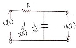
$$\frac{V_0'(s)}{V_1'(s)} = \frac{1}{K(s)} = \frac{1}{1+sRC}$$
