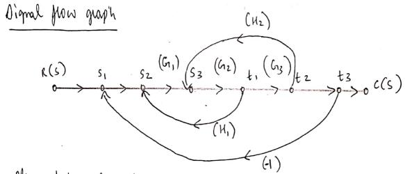
No. of forward paths = 1  $T_1 = 1 \times 1 \times G_1 \times G_2 \times G_3 \times 1 \times 1 \times 1 = G_1 \cdot G_2 \cdot G_3$
