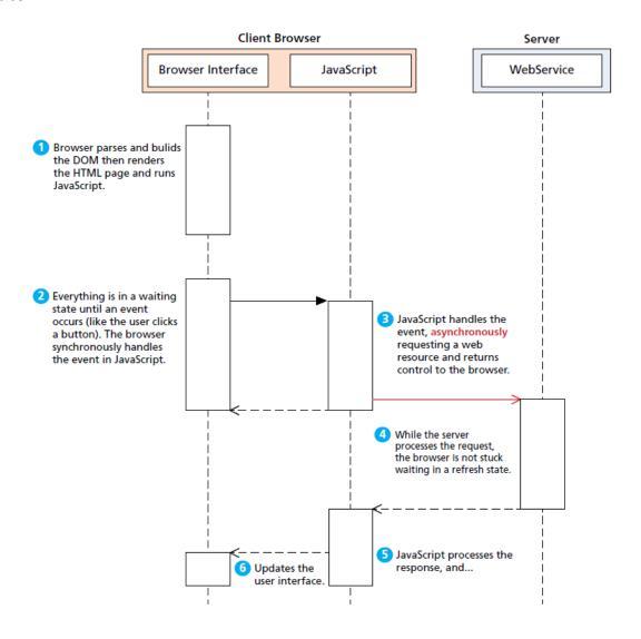
Figure 1: UML sequence diagram of an AJAX request
