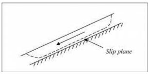
• Translation failure occurs in the case of infinite slopes and here the failure surface is parallel to the slope surface.
