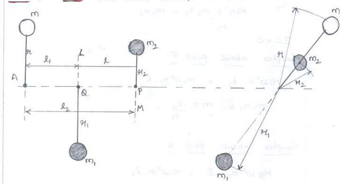
Consider a disturbing mass on lying in plane A to be balanced by two notating masses on, & m2 lying in different planes L & M as shown.
