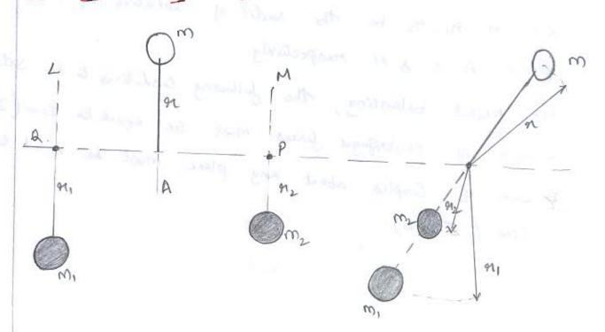
Consider a disturbing mass 'n' lying in plane A to be planned by two notating mass in mass m, & m2 lying on either side in different plans L& M as shown. Let m, n, n, n, be the radii of rotation of masses in planes A, L& M respectively.
