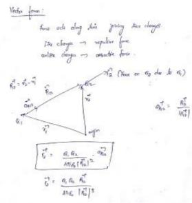
(b) A charge  $Q_A$  of -20 $\mu$ C is located at A (-6,4,7) and a second charge  $Q_B$  of 50  $\mu$ C [04] CO1 L3 is located at B(5,8,-2). Find force on  $Q_B$  due to charge  $Q_A$ . Assume both the charges are placed in free space.
