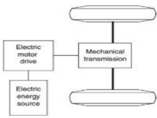
FIGURE 4.1 Primary electric vehicle power train
