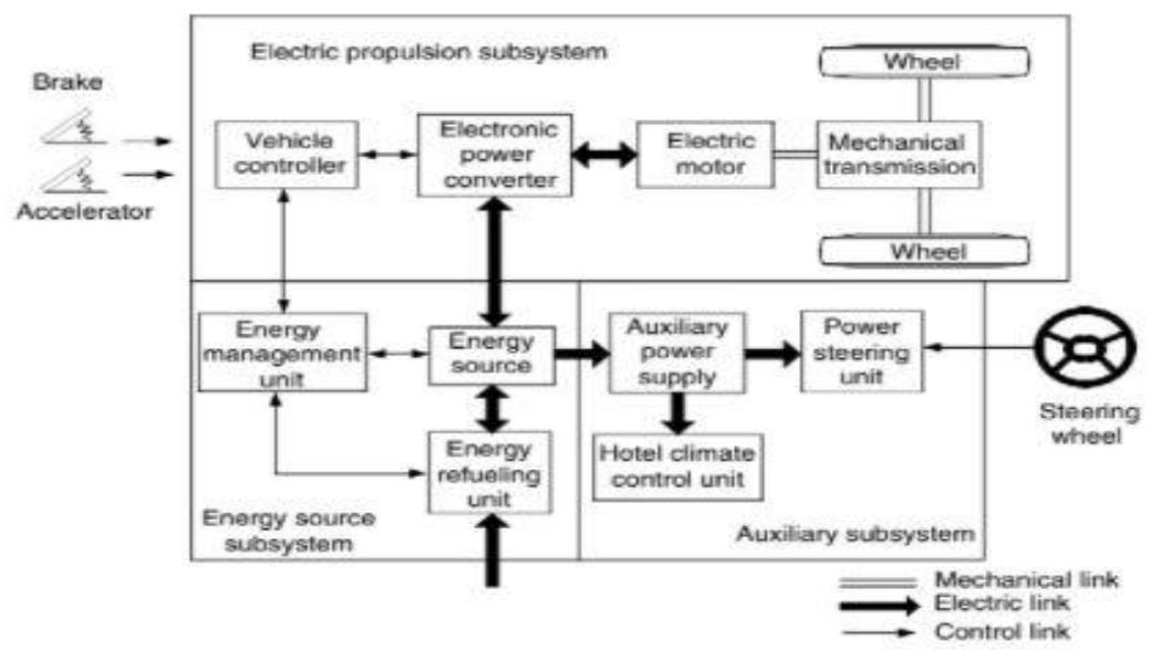
FIGURE 4.2 Conceptual illustration of general EV configuration.
