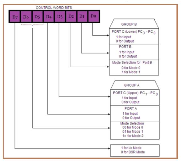
The control word to configure all the ports as output is given below.
