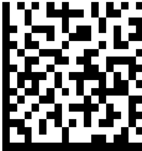
Figure 12.7 A 2-D matrix bar code. Shown is an example of the Data Matrix symbol.
