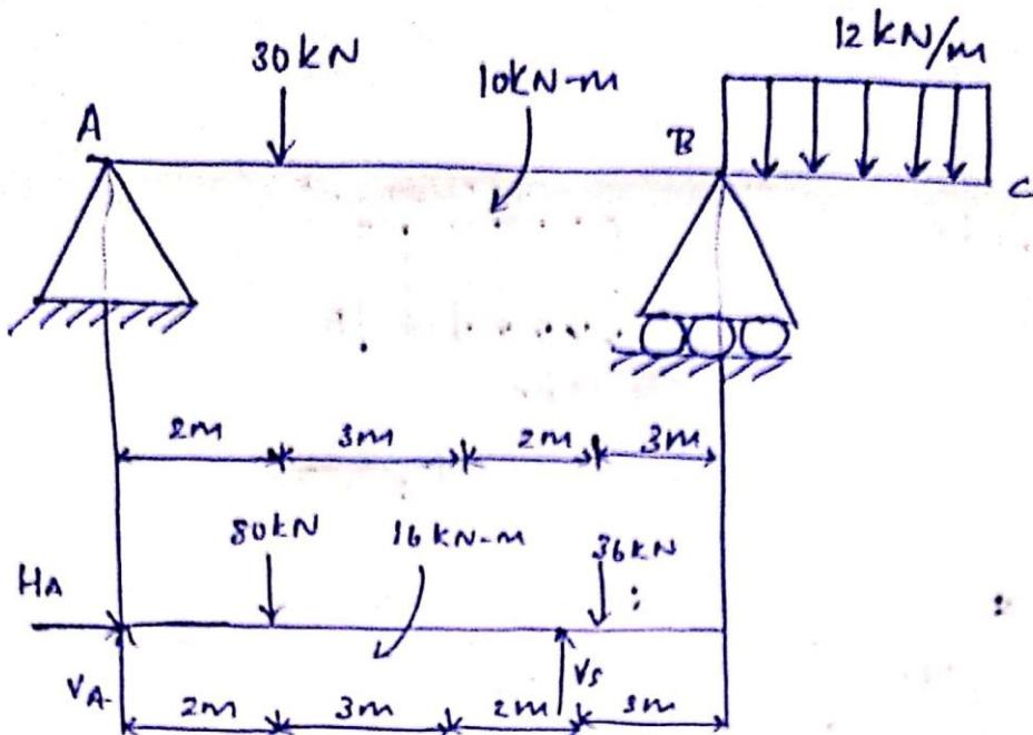
Converting UDL to point load
