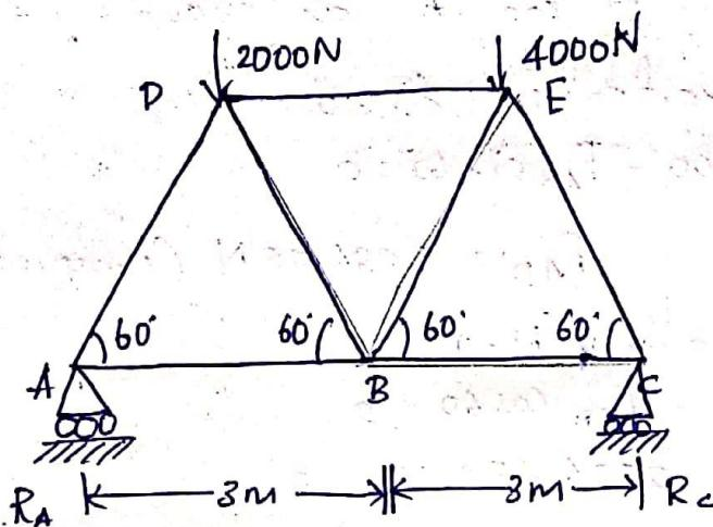
Solu Let  $R_A$  and  $R_C$  be the reactions at A and C respectively.
