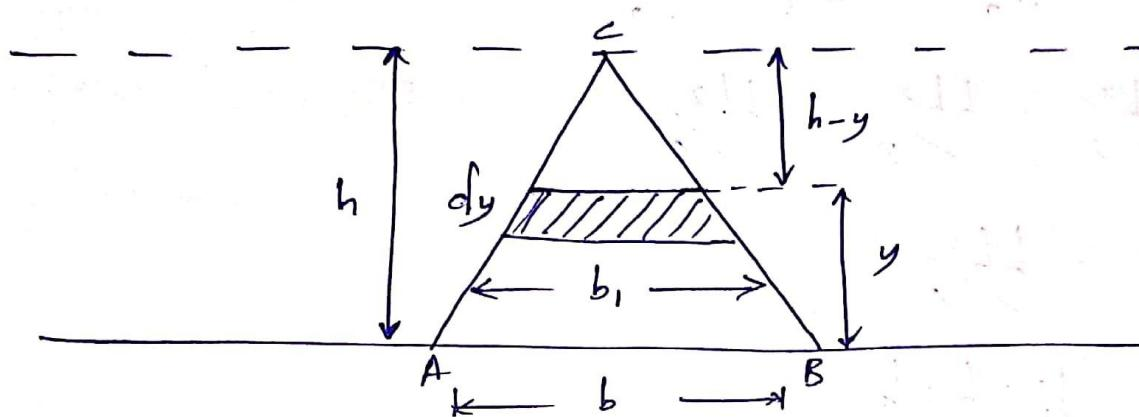
Now consider an elemental stripe of area  $\delta \cdot (b_1 \times dy)$  at a distance of  $y$  from AB (Base). Using property of similar  $\Delta$ 's,
