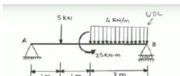
4 (a) Determine the support reactions of the beam as shown in below figure. [02]
