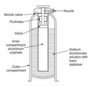
Portable extinguishers expelling foam are recommended for class B fires involving flammable liquids like oils, solvents, petroleum products, varnishes, paints, etc. The foam expelled by actuating the extinguishers forms a blanket over the surface.
