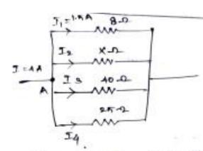
Voltage across. 80, resistor = IR = 1.5x8 = 12 V.
