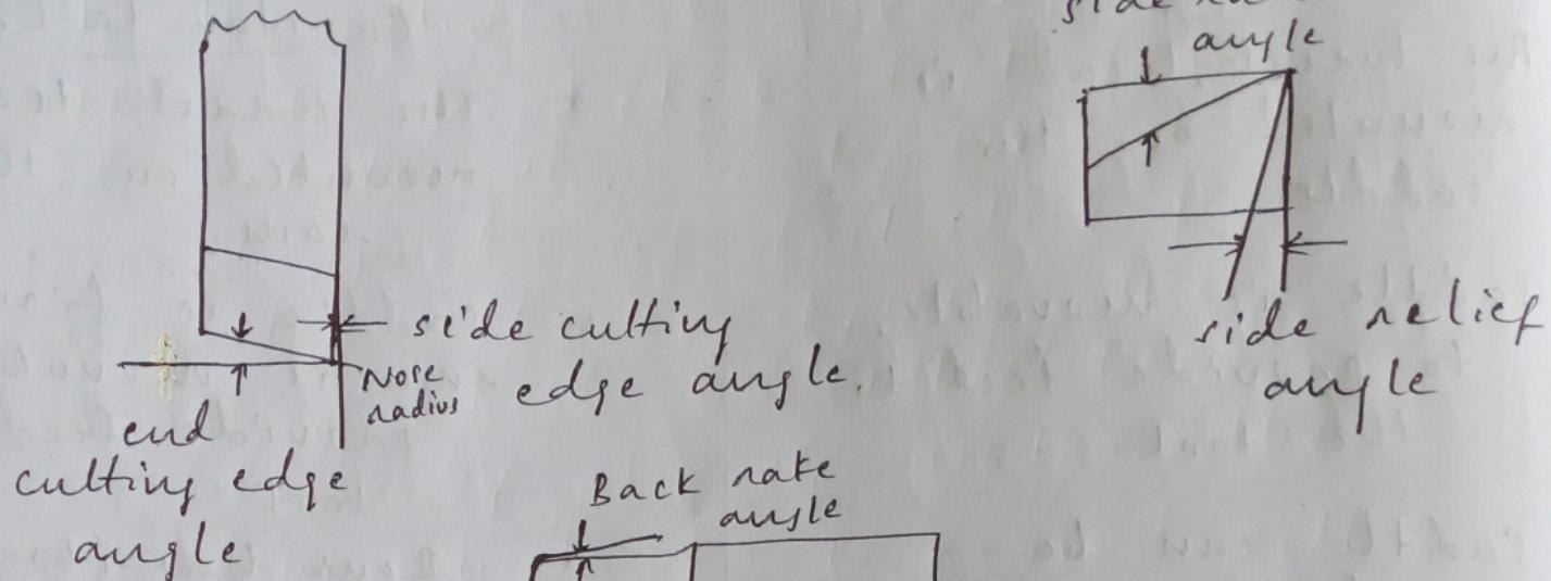
$$\text{Back rake angle} = 10^\circ$$
