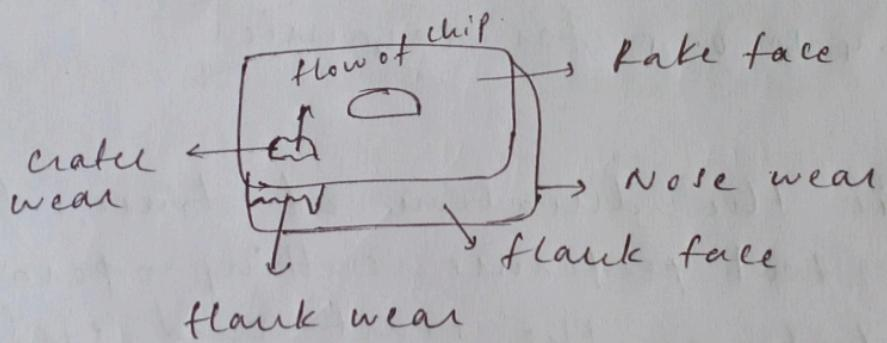
Flank wear :- The gradual and progressive wear on the flank portion of the cutting tool is called flank wear. It is a band gets formed on the surface of the tool due to continuous rubbing of machine part of the workpiece. The width and
