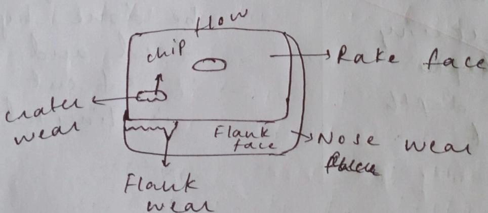
Flank wear:- the gradual and progressive wear on the flank portion of the cutting tool is called flank wear. The land gets
