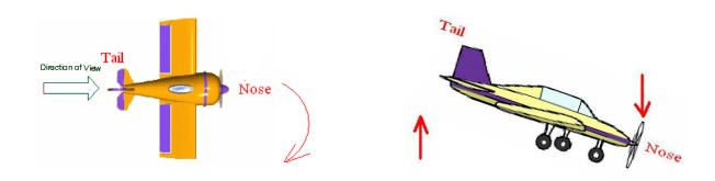
2. When the engine or propeller rotates in **anticlockwise** direction when viewed from the **rear** or tail end and the aeroplane takes a **left** turn, then the effect of reactive gyroscopic couple will be to **dip the nose** and **raise the tail** of the aeroplane.
