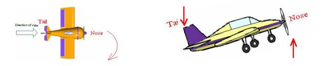
4. When the engine or propeller rotates in **clockwise** direction when viewed from the **front** and the aeroplane takes a **left** turn, then the effect of reactive gyroscopic couple will be to **raise the tail** and **dip the nose** of the aeroplane.
