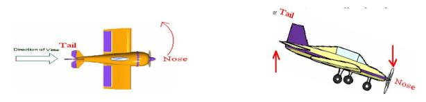
3. When the engine or propeller rotates in **anticlockwise** direction when viewed from the **rear** or tail end and the aeroplane takes a **right** turn, the effect of reactive gyroscopic couple will be to **raise the nose** and **dip the tail** of the aeroplane.
