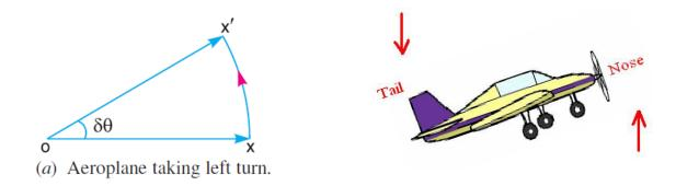
Effect of this couple is, to raise the nose and dip the tail of the aeroplane.
