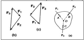
Figure (a) indicates an example for the three force member and (b) and (c) indicates the force polygon to check for the static equilibrium.
