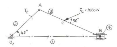
AC=70mm, AB=150mm, O<sub>2</sub>A= 40mm
